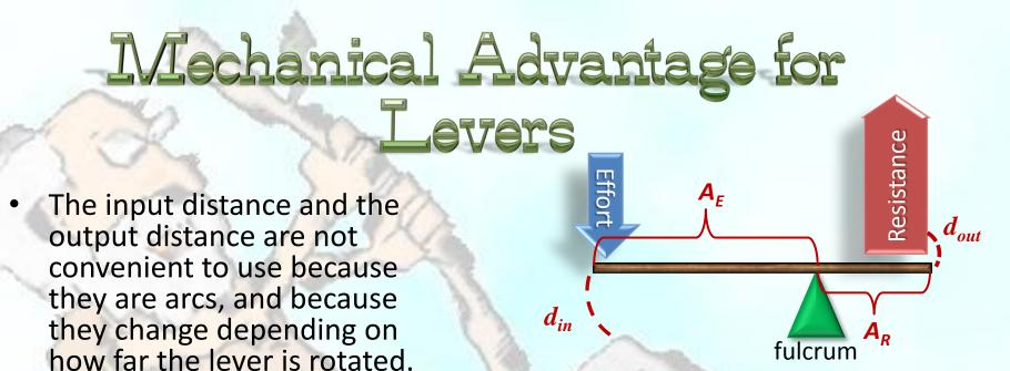
The input distance and the output distance stay proportional as the lever rotates, because their radii are the lever arms, and those are fixed lengths. (*NOTE*: The larger lever arm makes a larger circle as it rotates, and the smaller one makes a proportionately smaller circle.)
