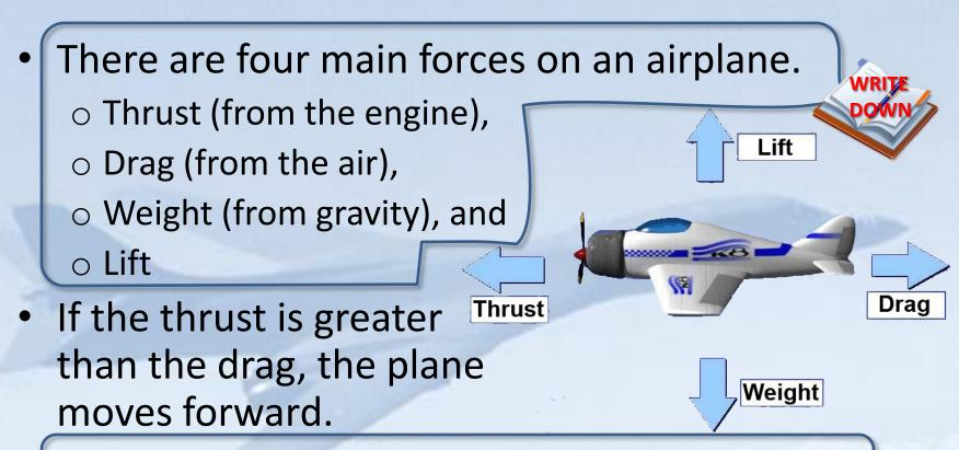
If the lift is greater than the weight, the plane moves upward.
