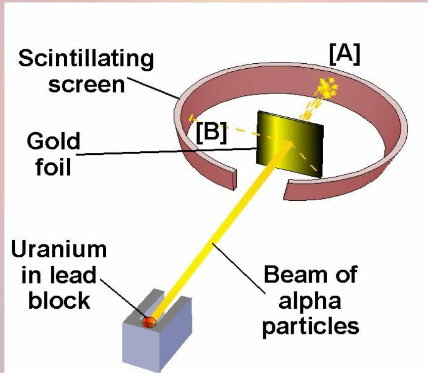
[A] Particles going through the foil [B] particles scattering
